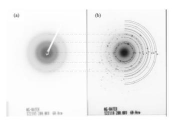
*Figure 3: Diffraction images from areas containing particles of dimensions: (a) nanometric, (b) micrometric.*
