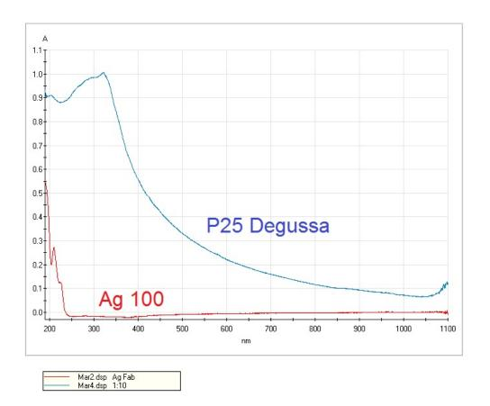
*Figure 5: UV/Vis absorption spectrum of colloidal silver Ag 100 (dispersion I) (red). For comparison, the absorption spectrum of typical photocatalyst, P25 Degussa (with the same concentration of TiO2 as colloidal silver Ag 100, i.e. 35 ppm) is also shown (blue).*
