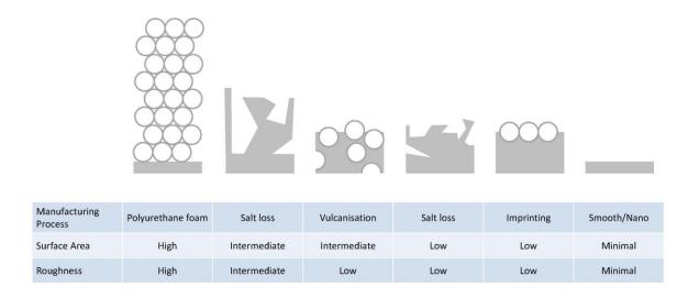
**Figure 1.** Implant surface texturing as it relates to the manufacturing method, surface area and surface roughness (based on Jones *et al.*, 2018).
