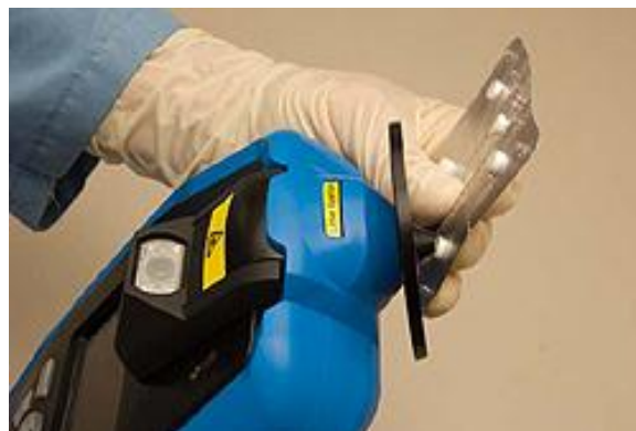
Figure 22 - Spectroscopy devices allow verification of chemical compounds (Source: www.ahurascientific.com )
