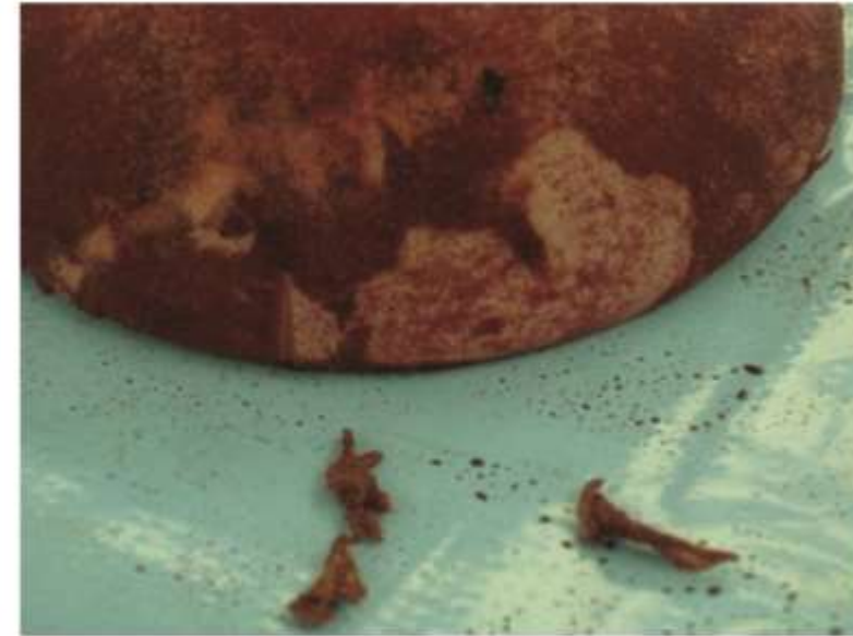
Figure 3. An early delamination of a polyurethane Silimed breast implant (courtesy of Daniel Fleming, MD, Brisbane, Australia).
