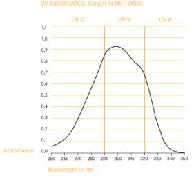
Specific extinction E<sup>1%</sup>/<sub>1cm</sub>, in methanol at  $\lambda_{max}$  299  $\pm$  2 nm: min. 930
