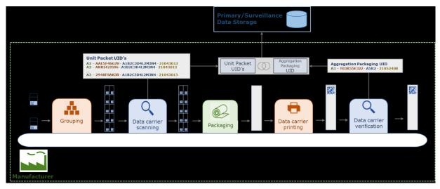
Figure 26: Aggregation processes and linkage of unique identifiers
