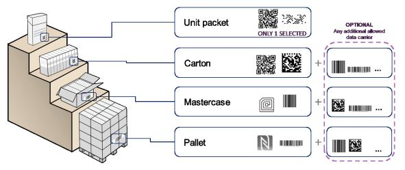
Figure 15. Description of the system with limited variety of data carriers per identification level and optional data carriers for aggregation packaging levels
