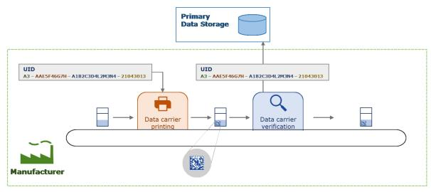
Figure 21: Unique identifier authentication at unit packet level
