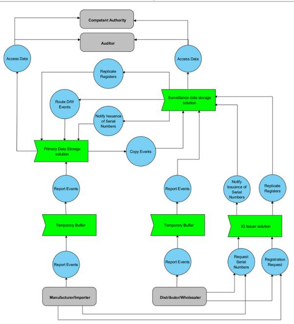
Figure 36: Tracking and Tracking main data flows
