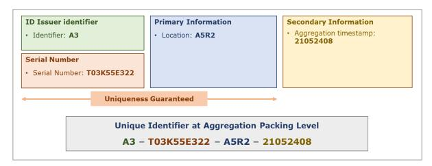
Figure 23: Composition of the unique identifier at aggregation packaging level
